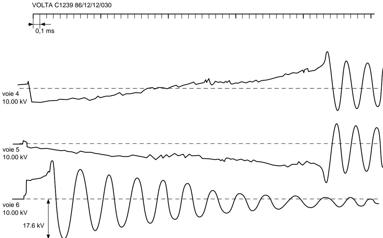
fig. 15: 3 phase interruption of 100 A with FG2 CB at 7.3 kV with IEC motor substitute circuit.
