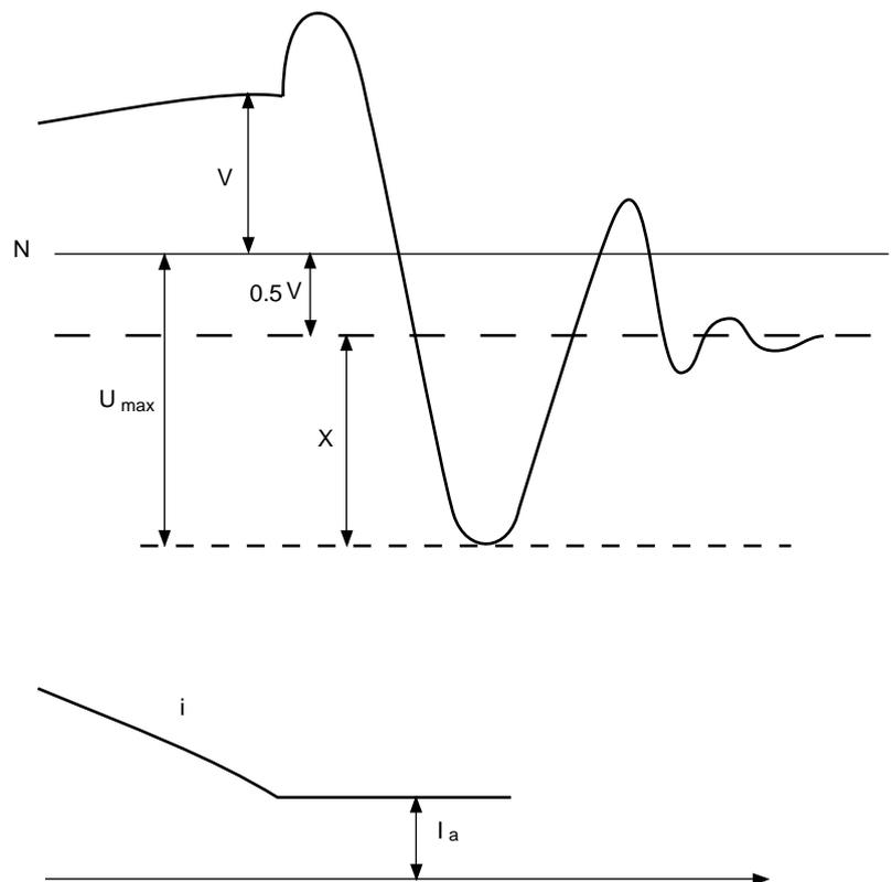
fig. 13: interruption of the first phase with current chopping  $I_a$ .
