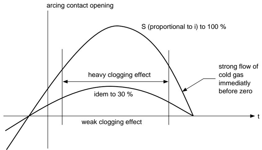
fig. 3: variation of the arc cross sections at 30 % and 100 % of the breaking capacity.
