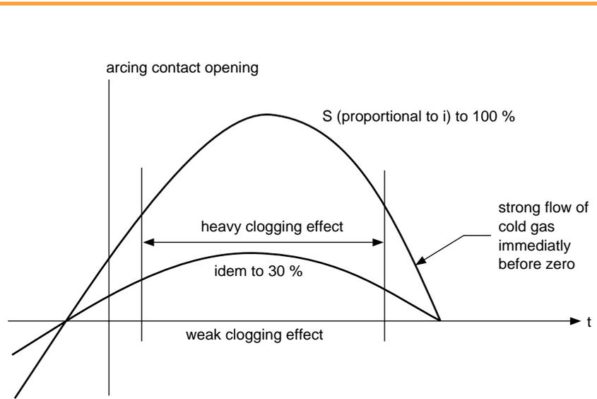
fig. 3: variation of the arc cross sections at 30 % and 100 % of the breaking capacity.
