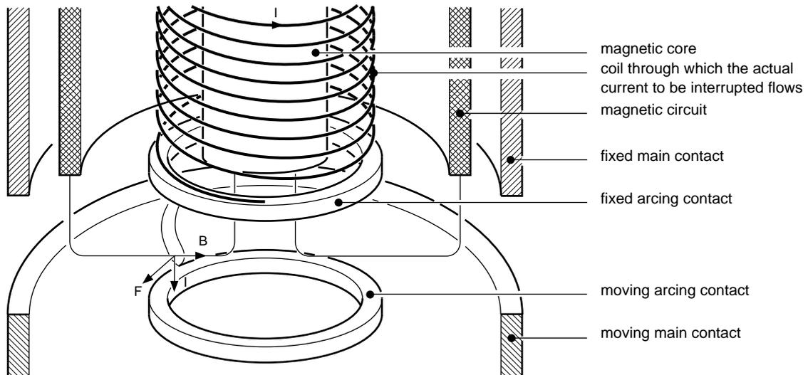
fig. 5: example: rotating arc contactor (Rollarc).
