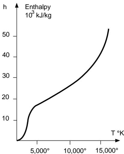
fig. 1: enthalpy of SF6 as a function of temperature.
