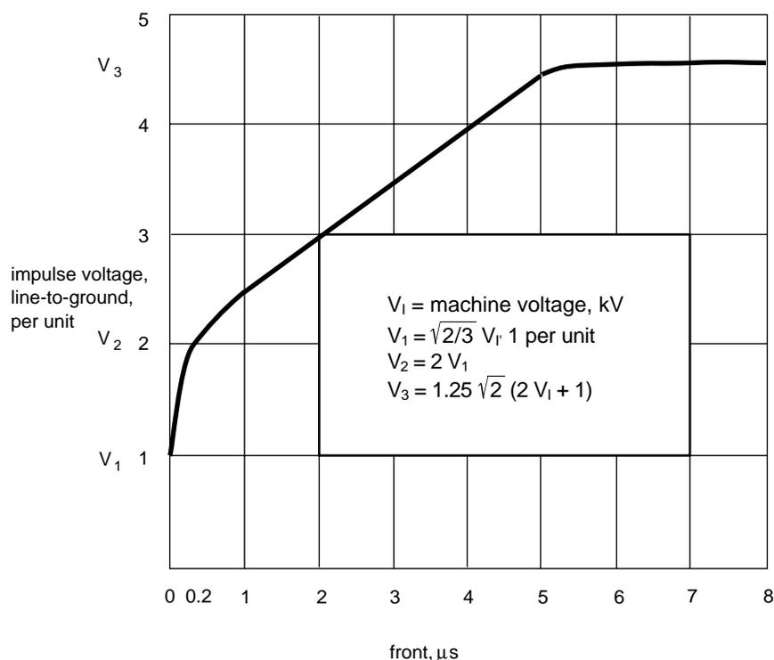
fig. 9: machine impulse voltage withstand envelope.
