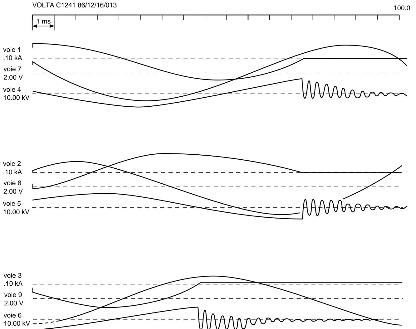
fig. 16: 3 phase interruption - 100 A with FG1 7.3 kV without current chopping.
