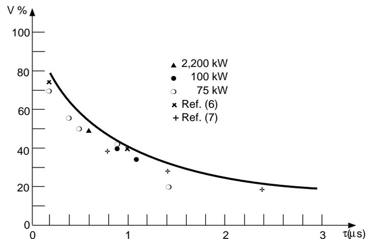
fig. 8: % of wave front magnitude as a function of wave front time.
