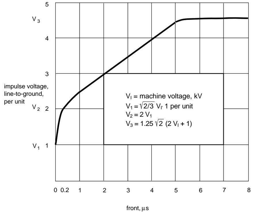
fig. 9: machine impulse voltage withstand envelope.
