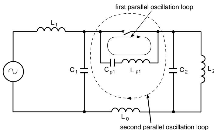
fig. 11: equivalent circuit
