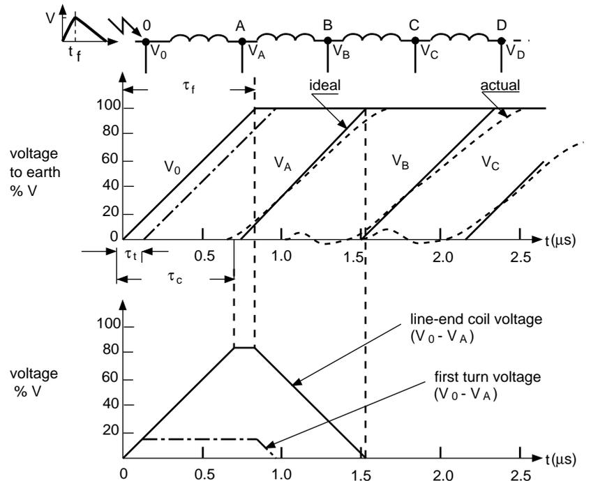
fig. 7: interturn and intercoil voltages developed in a winding subject to steep fronted voltage transients (time in microseconds).
