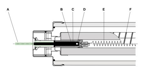
Fig. 14: example of a thermal trip unit incorporated into the striker system of all Merlin Gerin brand fuses. A. striker released
