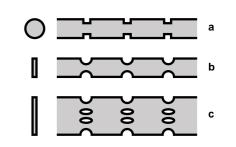
Fig. 12: fuse elements with sections of varying sizes.
