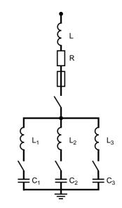
*Fig. 23:* diagram of a bank with three capacitor steps protected by a single fuse.
