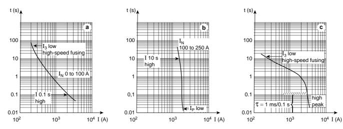
Fig. 25: ideal time/current characteristics for protecting:
