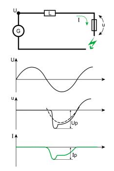
Fig. 3: diagrams showing disconnection at I1.
