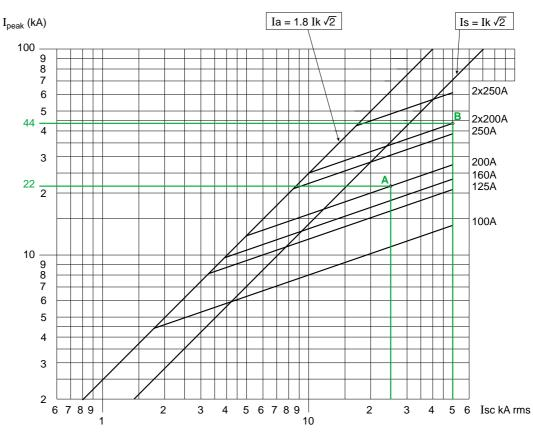
Fig. 27: current limitation curves according to rating (Fusarc-CF, Merlin Gerin brand).
