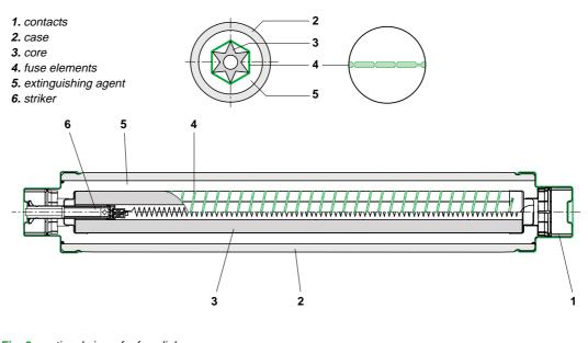
Fig. 8: sectional view of a fuse link.
