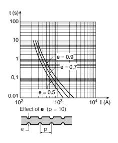
Fig. 11: effects of notching on a fuse element.
