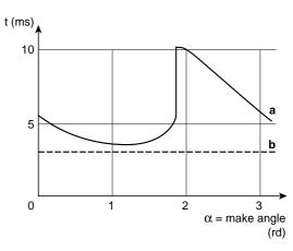
*Fig. 6:* actual (*a*) and virtual (*b*) pre-arc durations on a Fusarc-CF 25 A (Merlin Gerin).
