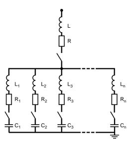
Fig. 22: diagram of a multiple step capacitor bank.
