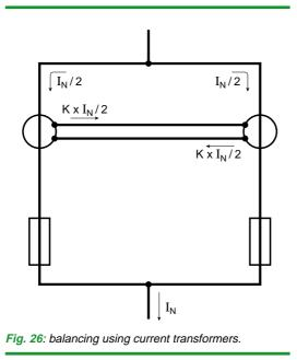
assembly comprising two parallel links rated at 200 A will have an  $I_N$  of: 2 x 200 x 0.8 = 320 A.  $\Box$  I1: although in theory installing n links in parallel should enable the I1 of the assembly to be multiplied by n (each element only being traversed by  $I_N / n$ ), in reality, this type of calculation is extremely dangerous as the slightest fault on one link will jeopardize the operation of the assembly.
