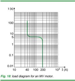
This current,  $I_{\text{S}}$ , which is known as the starting current or the locked rotor current, is quantified by the ratio  $I_{\text{S}}/I_{\text{N}}$ , which is typically equal to 6 in the case of direct on-line starting.
