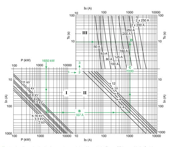
Fig. 19: chart illustrating the time/current characteristics of fuses in the Fusarc-CF (source Merlin-Gerin) range.
