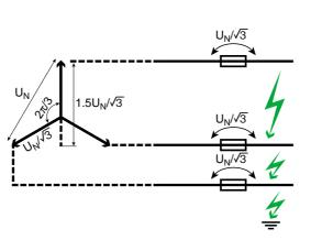
Fig. 2: voltage at the fuse assembly terminals in the event of a three-phase fault on an isolated neutral system.
