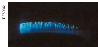
Fig. 3: diffuse vacuum arc AMF technology
