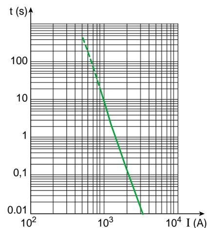
**Fig. 4:** pre-arc duration as a function of the rms current value.
