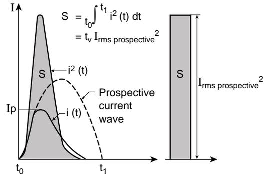
**Fig. 5:** chart indicating the virtual duration of the pre-arc.
