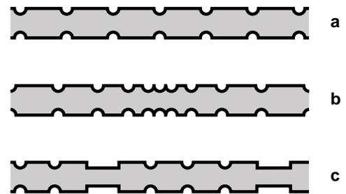
**Fig. 13:** different types of notching.
