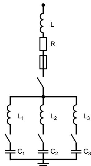
Fig. 23: diagram of a bank with three capacitor steps protected by a single fuse.
