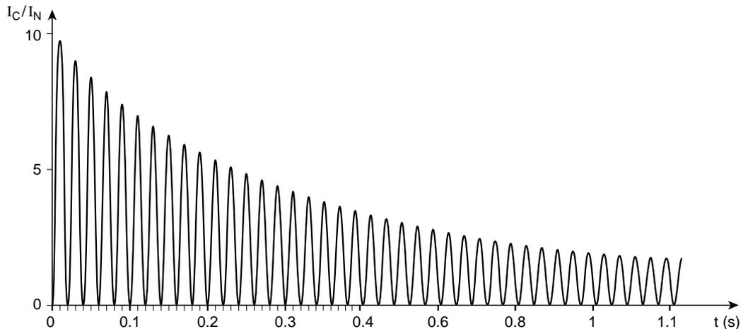
**Fig. 15:** maximum inrush or peak current of a 1 000 kVA transformer.
