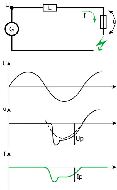
**Fig. 3:** diagrams showing disconnection at I1.
