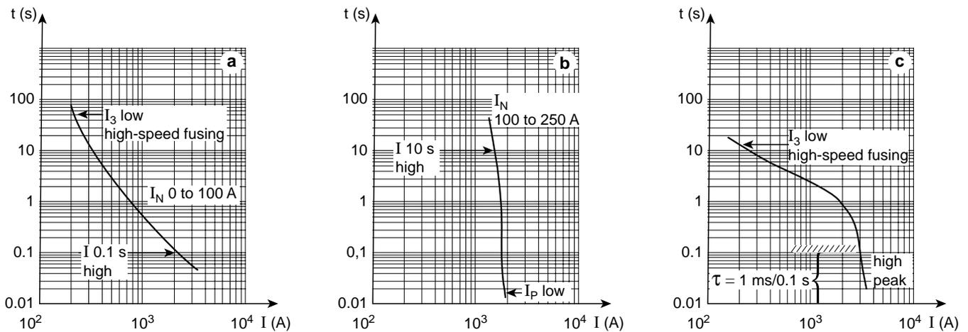
Fig. 25: ideal time/current characteristics for protecting:
