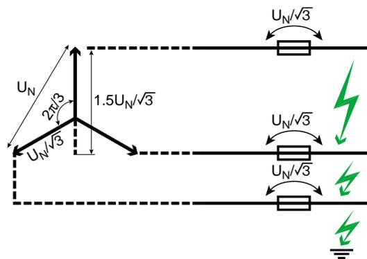
**Fig. 2:** voltage at the fuse assembly terminals in the event of a three-phase fault on an isolated neutral system.
