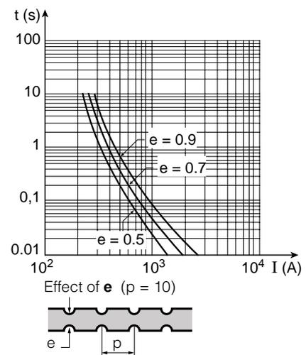
**Fig. 11:** effects of notching on a fuse element.
