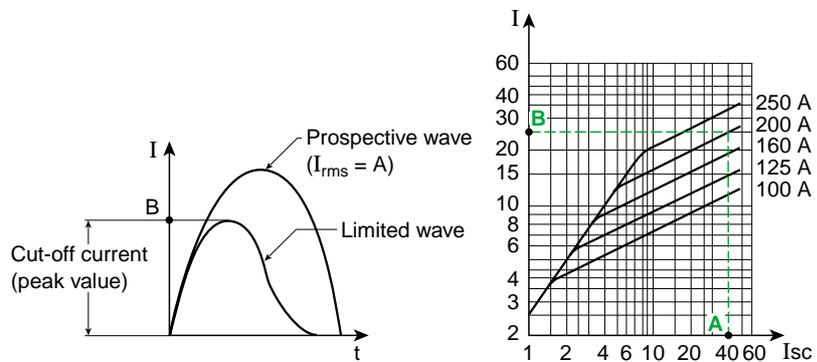
**Fig. 7:** value  $I_p$  of the limited cut-off current as a function of the prospective current.
