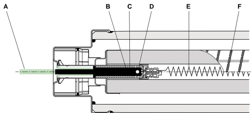
**Fig. 14:** example of a thermal trip unit incorporated into the striker system of all Merlin Gerin brand fuses.
