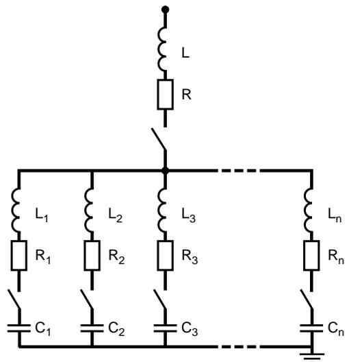
**Fig. 22:** diagram of a multiple step capacitor bank.
