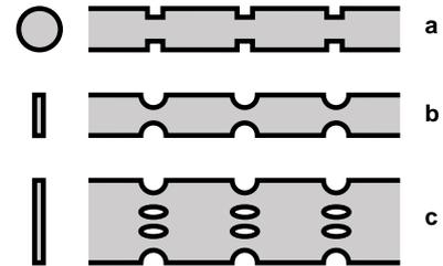
**Fig. 12:** fuse elements with sections of varying sizes.
