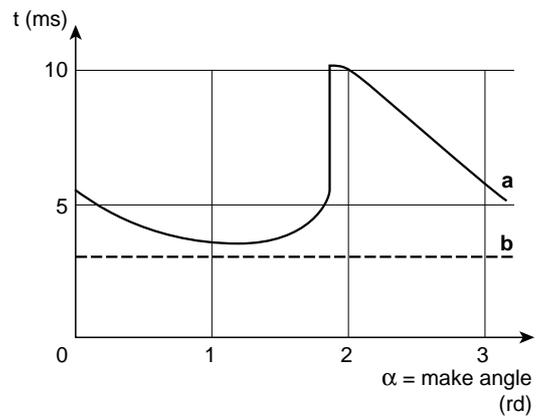
**Fig. 6:** actual (a) and virtual (b) pre-arc durations on a Fusarc-CF 25 A (Merlin Gerin).
