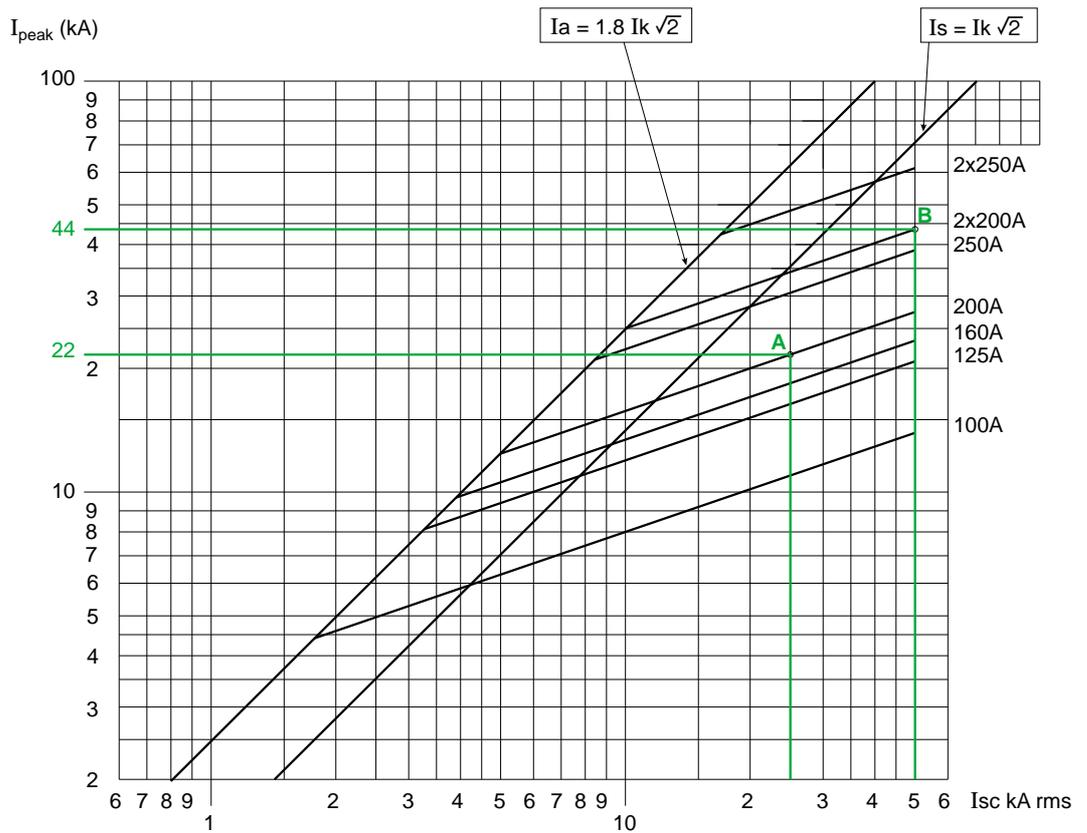
Fig. 27: current limitation curves according to rating (Fusarc-CF, Merlin Gerin brand).
