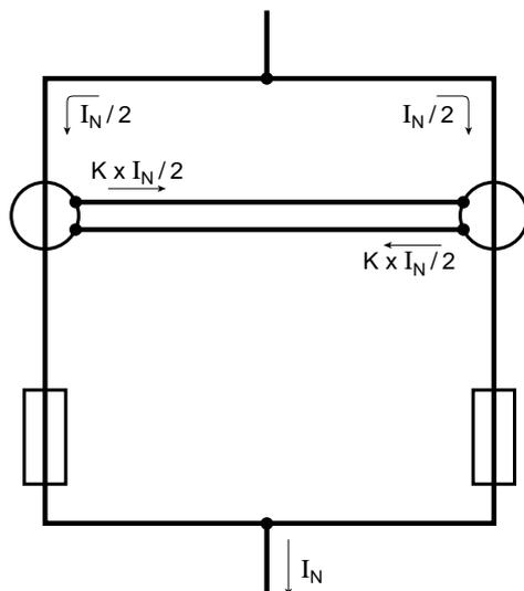
**Fig. 26:** balancing using current transformers.
