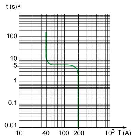
**Fig. 18:** load diagram for an MV motor.
