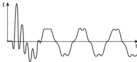
**Fig. 21:** transient current wave on starting a capacitor bank.
