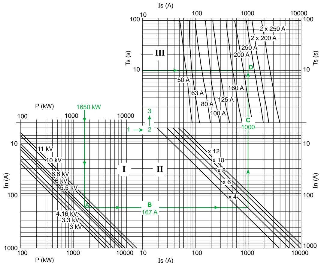
Fig. 19: chart illustrating the time/current characteristics of fuses in the Fusarc-CF (source Merlin-Gerin) range.
