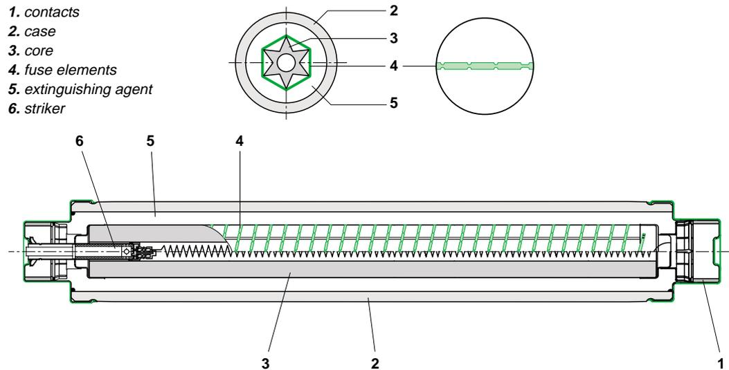
**Fig. 8:** sectional view of a fuse link.
